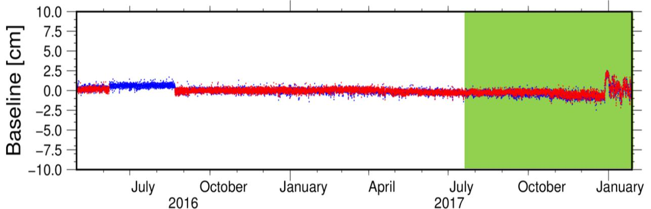
Figure 5.1.1: Relative distance changes between GDS2 and GDS5 (compare Fig. 3.1.2) for the entire observation period. Green background marks the new data obtained during this cruise.
